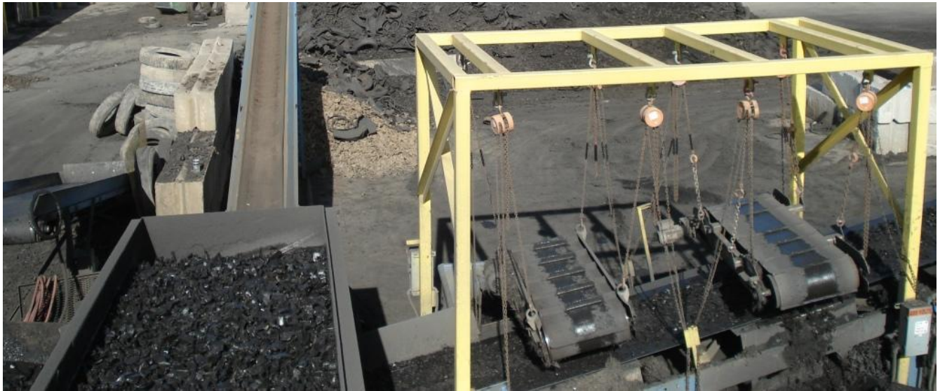
Two belt magnets to the right of the picture removed loose wire at Liberty Tire in Jefferson County. Liberty Tire is the largest supplier of tire derived products in the Commonwealth. (Photographs courtesy of Terry Gray, TAG Resource Recovery, November 2012).
